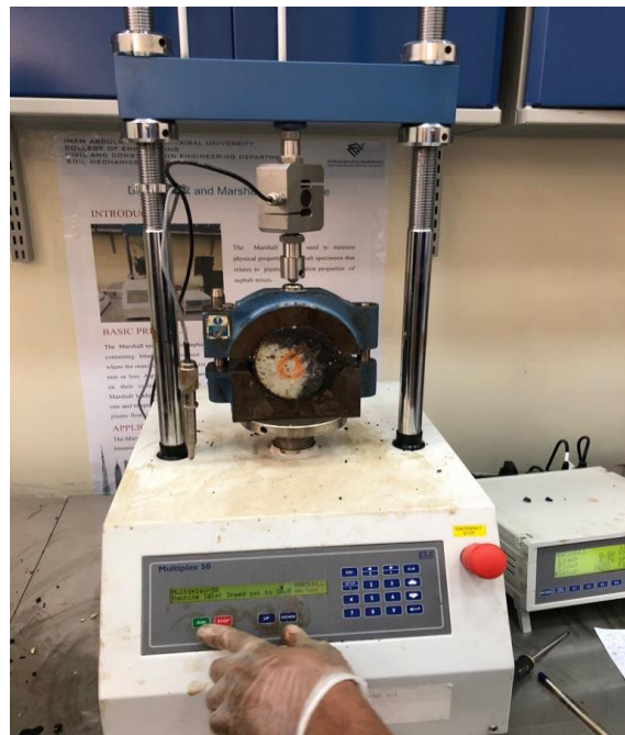
Figure 2: Marshall test to obtain optimum bitumen content
