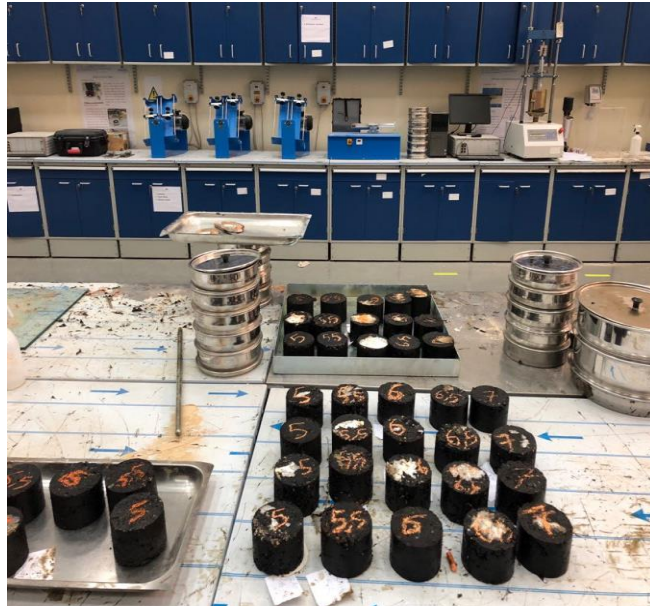
Figure 1: Mix design preparation using different aggregate types
