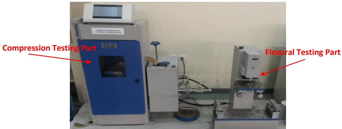
Fig. 2: Compression and Flexural Testing Machine
