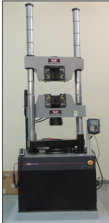
Figure 12: Universal Testing Machine (UTM)
